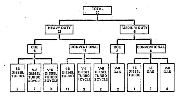
Figure 5-1. TEST VEHICLE CONFIGURATIONS
