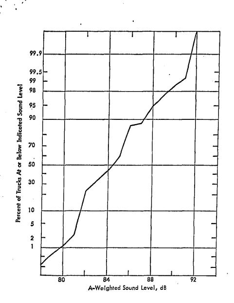
Figure 5-45. Cumulative Distribution of New Diesel Truck Noise Levels (372) (Reference 35)
