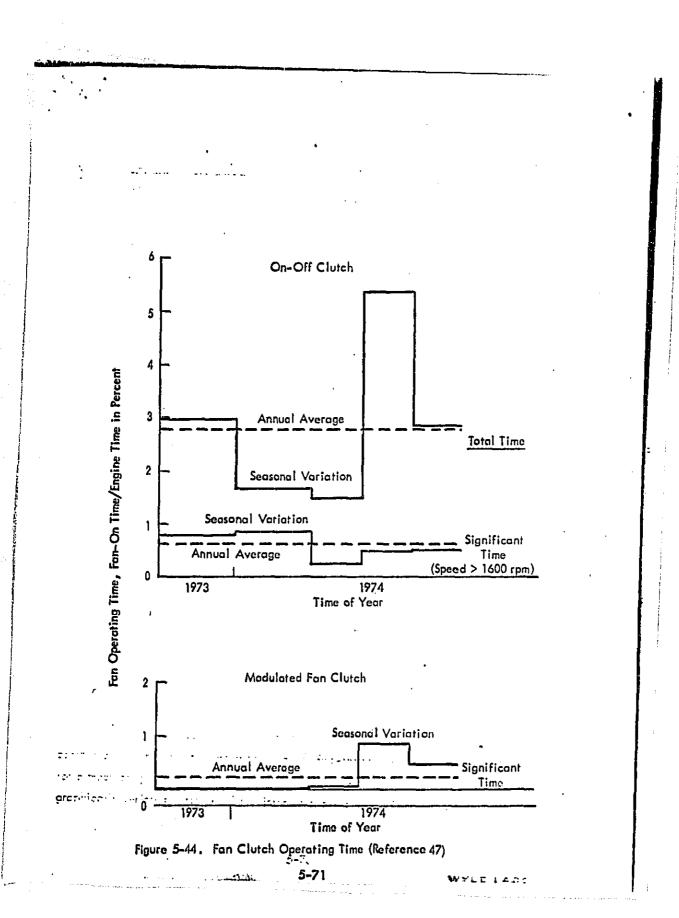
The data shown in Figure 5-44 were accumulated for the on-off clutches by using elapsed time meters on the engine and fan clutch. A multichannel tachograph was also used to monitor engine rpm and provide an event marker indicating clutch engagements. The top curve represents the total fan-on time as a percentage of engine-on time. The lower curve depicts fan-on time occurring above 1600 rpm, which is "significant fan-on time" by definition.
